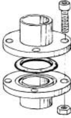
Figure 3: Exploded view of a gasket seal.
